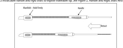
**Figure 2:** Handle and Rigid Shaft Retraction — Hold handle and manifold firmly while retracting rigid shaft. 3. Perform a "Pre-Freeze" by cycling the ACM using the activation button or footswitch while the PROBE is in air.
