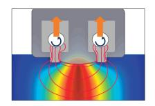
Conclusions: This irrigated bipolar radiofrequency probe consistently produced transmural lesions in tissue 4 mm or thinner under controlled conditions in vitro. Lesion depth was increased by greater pressure on probe and not affected by blood flow. Endocardial lesions were smaller than epicardial dimensions. \*Study based upon 5 mm tissue thickness
