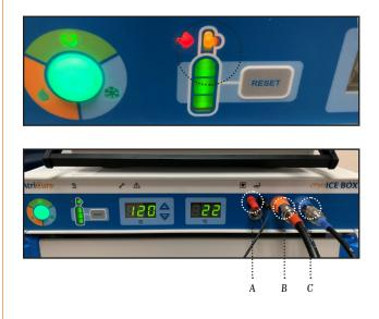
**Note:** Be sure to route the N<sub>2</sub>O vent tubing to a safe area prior to use.
