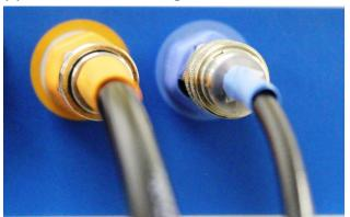
Figure 14: Color Coded Pneumatic Connectors
