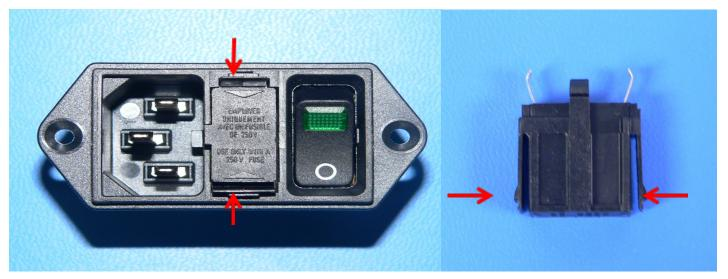
Figure 19: Fuse Box Tabs
