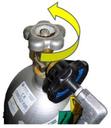
Figure 7: Turn Valve Counter-Clockwise to Open
