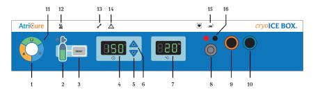
Figure 2: AtriCure Cryo Module Front Panel
