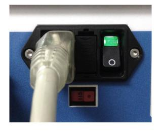
Figure 11: Turn-ON AtriCure Cryo Module with Switch
