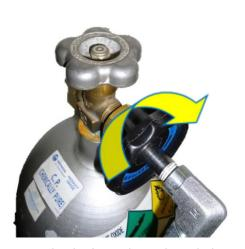
Figure 6: Attach Black Knob to Threaded Connection
