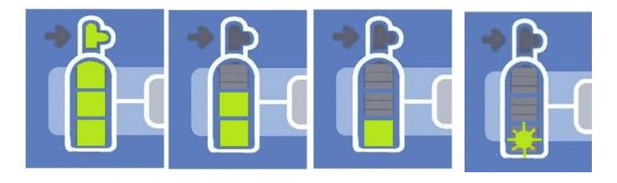
Figure 13: N<sub>2</sub>O Gauge Indicators
