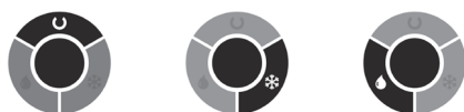
[a] Ready Mode (green) [b] Freeze Mode (blue) [c] Defrost Mode (orange)
