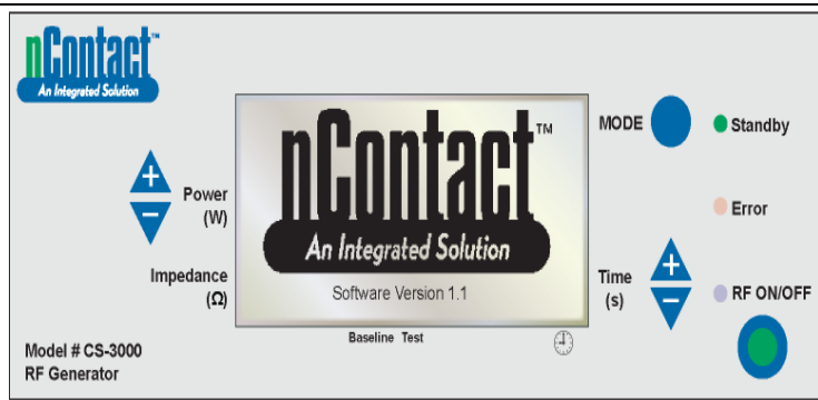
Figure 9. RF Generator Front Panel Display at “Standby Mode”
