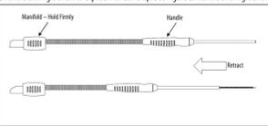
**Figure 2:** Handle and Rigid Shaft Retraction – Hold handle and manifold firmly while retracting rigid shaft.
